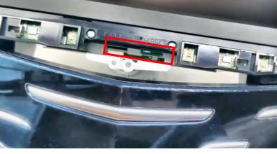
When placing the screen, try to get the alignment pins in first before tightening screws. If the alignment pins do not go in, the screen will not sit flat.
