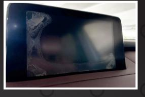
This one is a unique design that uses a plastic assembly that contains the cover glass, bezel, and digitizer. The replacement part was just released. These factory screens are at 100% failure rate from the factory. Customers save \$2,000 from the dealer. Incredibly easy to access the display and install.
