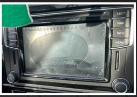
The MIB2 radio was put in almost every 2016+VW made, and the touch screen is now nearing the end of life. Sometimes it becomes frozen, sometimes the glue leaks out, etc. Depending on the customer preference and budget, you can install either one. Check the <u>info guide</u> to decide which is the right one for you.
