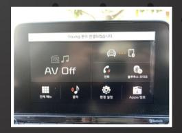
This screen lasts about 3 years from the factory, right outside of the electronics warranty from KIA. They used a very unfortunate LOCA design with a large, high torsion cover glass so all are guaranteed to fail. New head units are over \$3,000 from the dealer. We have the replacement screens, you disassemble the radio and heat the old assembly off the bezel.
