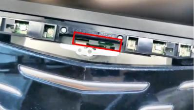
Route the ribbon through the unit using this large slot. Do not attempt to route through the small sharp metal opening below this, you will rip the cable.
