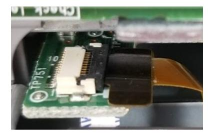
This is the correct ribbon installation. Fully inserted with the black side up, gold pins down toward the circuit board, and the large tab towards you. Make 100% sure this is how you have yours connected. Almost every time a customer has an issue with touch not working after screen replacement, it is due to not inserting the ribbon correctly.
